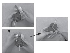
8. Reinstall the fences, making sure that the side blades lie parallel to the housing as they may slide down as they rotate around the back bushing — push them up before reinstalling the fences. Tighten. Also reinstall and firmly tighten the three Phillips screws securing the two halves of the housing.
