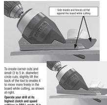
Operate your drill at its highest clutch and speed settings in DRILL mode. It is recommended that you use a 18V or higher-rated cordless or AC-powered drill.
