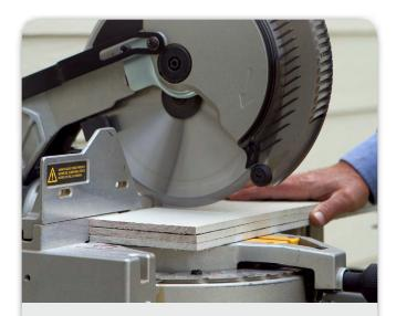
The original blade specifically designed for fiber-cement ripping and crosscutting
